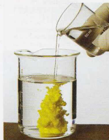
▲ Lead iodide precipitate is bright yellow.
