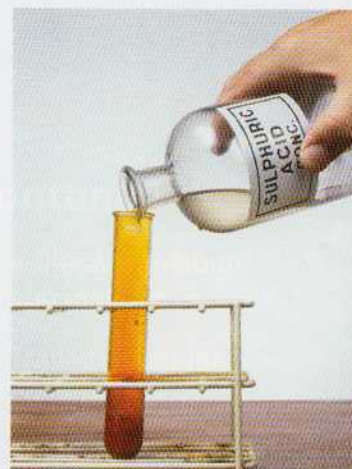
▲ The addition of concentrated sulfuric acid to sodium bromide.
