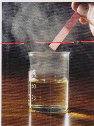
▲ Silicon chloride fumes in moist air as water reacts with it to release acidic HCl fumes.
